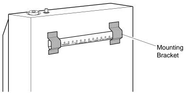
Figure 6 - Mounting Bracket
